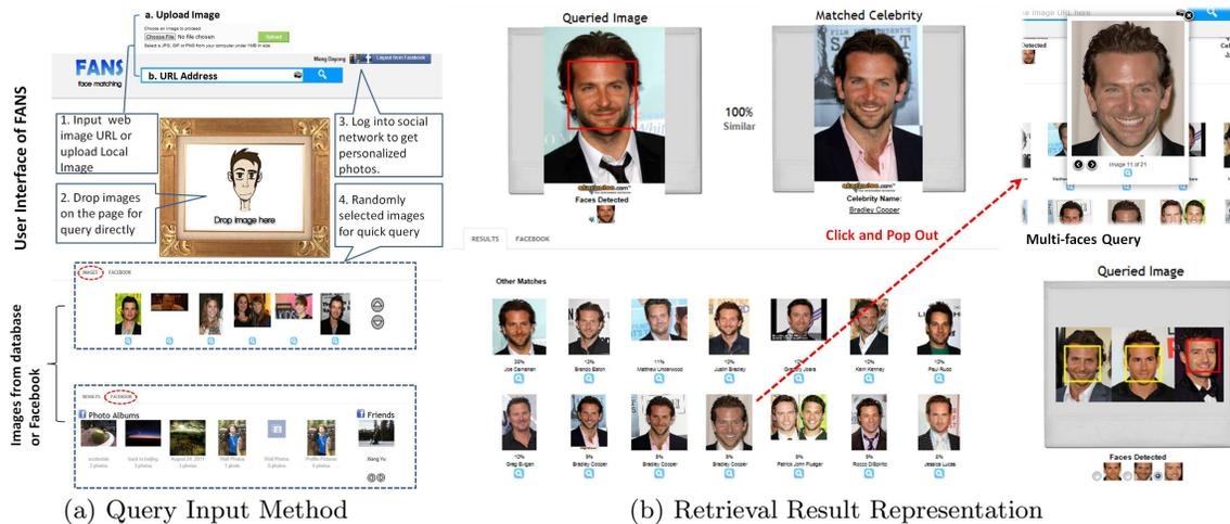
**Figure 2: The user interface of the FANS system. (a) The methods of inputting query facial image, including entering the URL, uploading the local image, and directly dragging the images on the webpage; (b) The representation of retrieval result.**
