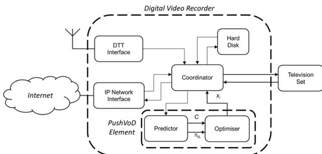
Figure 5: Schematic of a DVR/STB with SCORE
